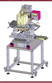
United Silicone's Peripheral Hot Stamp & Heat Transfer machine is used for peripheral application of heat transfer decals or decorative foils to cylindrical or tapered parts.
